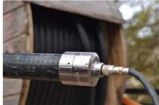
Figure 5: Connection between RF cable and RF flexible tail
